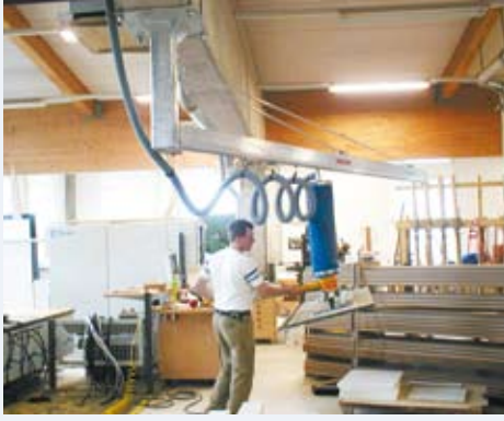
Slewing jib with ceiling suspension
