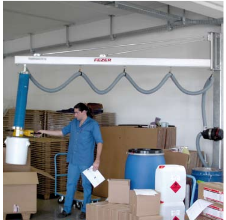
Column slewing jib for the handling of barrels
