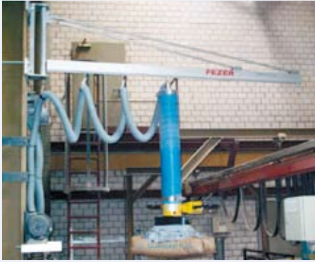
Wall slewing jib for sack handling
