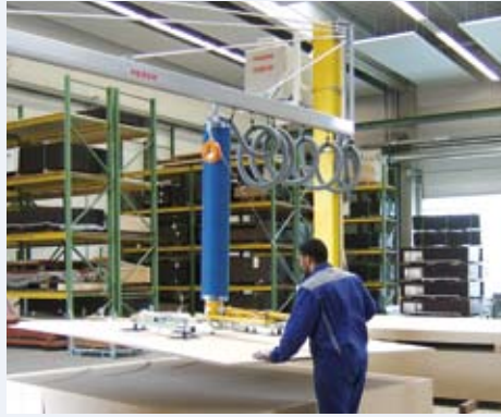
Slewing jib with long jib arm and fourfold suspension
