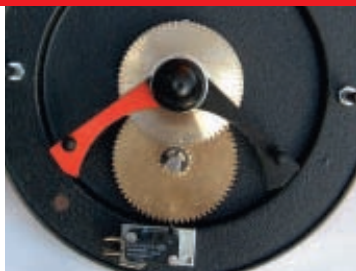
Upper and lower limit switch - Easy to set and very reliable.
