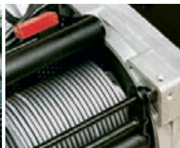
Rope press roll - This is the essential counterpart to the grooved drum.
