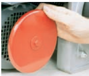
Trouble shooting hand wheel with brake release - Allows, without current, to lower or position a load.
