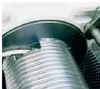
Grooved drum - Essential to install a 2 ways system.
