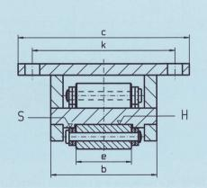
Mod. AS-H<sub>.</sub> (H = hardened and machined centre plate), AS-H-50CrV4 (roller material 50CrV4)
