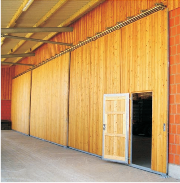
Sliding door system with multiple leaves, adjustable wall brackets for three tracks, adjustable support brackets and double wheel hangers, and integrated pedestrian door.
