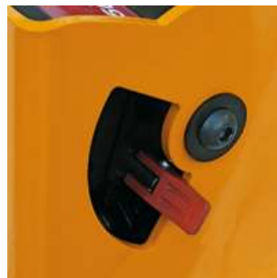
△ Drum release impossible when in load (except VS 250/320 without drum release).
