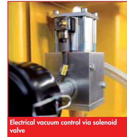
Switching automatic with automatic suction and release on setting down
