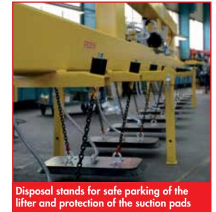
Disposal stands for safe parking of the lifter and protection of the suction pads
