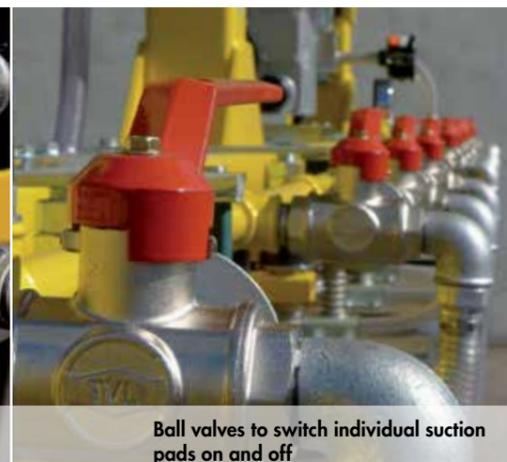
Ball valves to switch individual suction pads on and off
