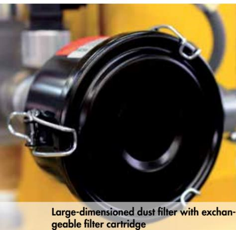
Large-dimensioned dust filter with exchangeable filter cartridge
