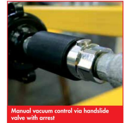
Manual vacuum control via handslide valve with arrest
