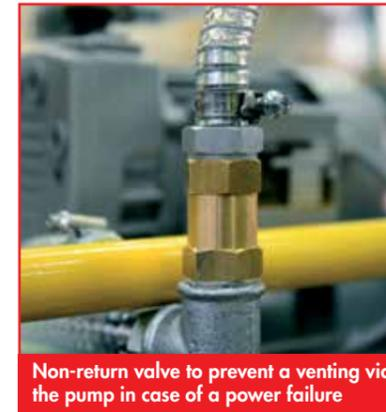
Non-return valve to prevent a venting via the pump in case of a power failure
