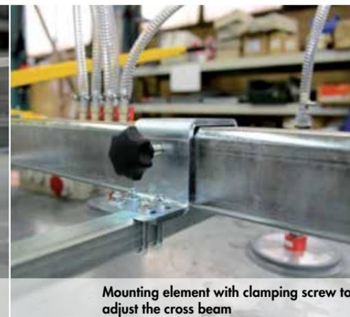
Mounting element with clamping screw to adjust the cross beam
