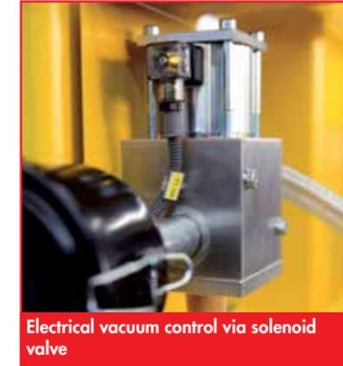
Electrical vacuum control via solenoid valve
