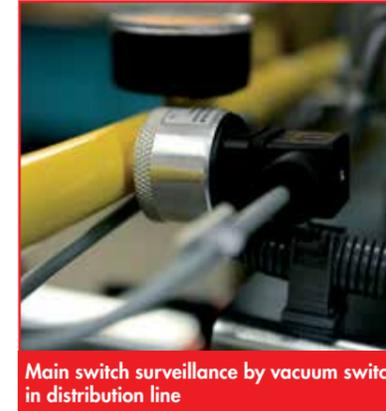
Main switch surveillance by vacuum switch in distribution line
